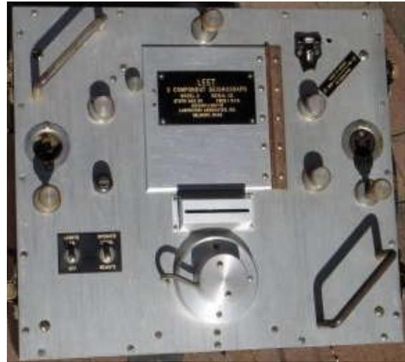
3 outer knobs are for leveling. 3 inner knobs are pendulum locks. Door is for film cannister.
