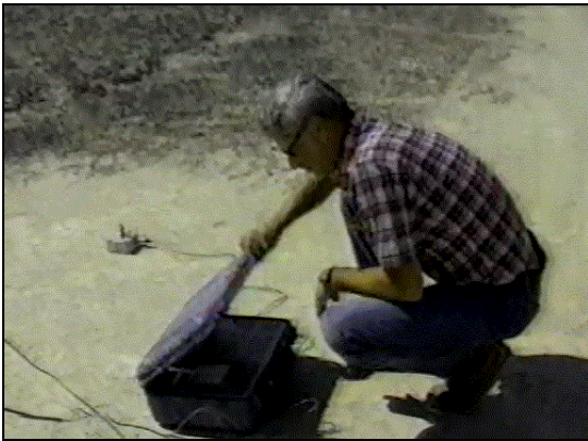
Checking to see what we've got on the conventional blasting seismograph.
